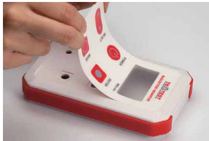
8. Sticking overlay sheet onto enclosure
